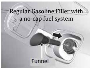
Regular Gasoline Filler with a no-cap fuel system
