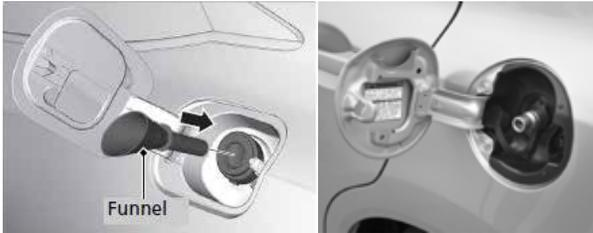
Regular Gasoline Filler with a no-cap fuel system
