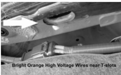
Bright Orange High Voltage Wires near T-slots
